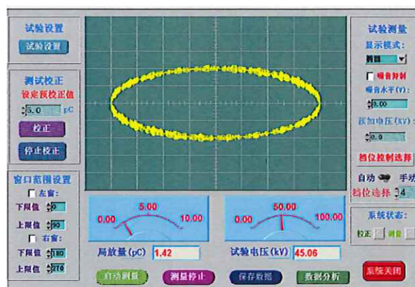
A2: 试验回路1红芯在45kV下局部放电试验图形 The oscillogram of partial discharge of red core at 45kV on test loop 1
