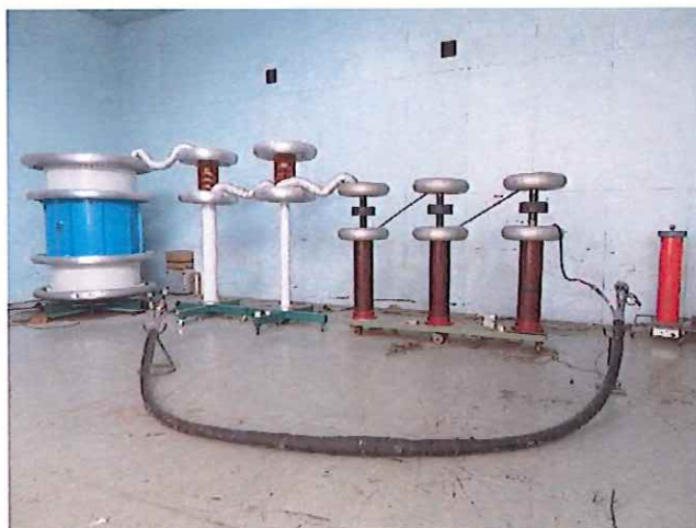
C2: 样品交流电压试验 AC voltage test on the sample
